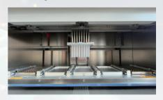
Disposable sheath insulates magnetic rods and samples, and machine is equipped with UV sterilization and air filtration systems to reject cross contamination adsorption
