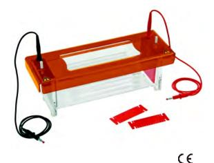
The Super plus is a compact system capable of running a maximum 1200 samples simultaneously by stacking up to 4 horizontal gels. This achieves high sample throughput while maintaining the time- and space-saving advantages of a small, compact unit.
